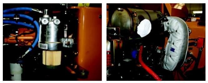
To protect the engines from damage due to water or dirt in the diesel fuel, Tigercat engineers spec'd a Racor GreenMAX fuel filter/water separator (left) for new machines. Custom-fit Firwin insulation blankets (right) help isolate hot spots in the engine compartment of this 845D feller buncher.
