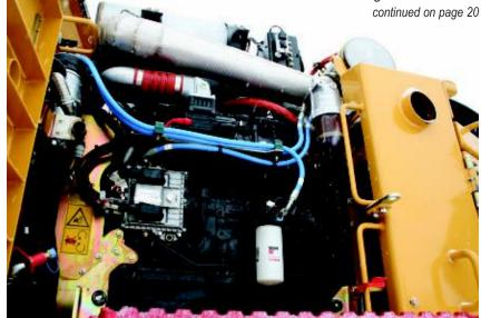
The 845D feller buncher uses a Tier 4 final FPT Industrial NEF N67 diesel engine rated 282 hp at 2200 rpm. The red platform at the bottom of the photo is included on machines with leveling undercarriages to help make regular maintenance safer and easier.
